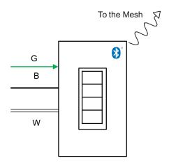
Dimmer #2 This Dimmer is wirelessly connected to Dimmer #1 and controls the load via Dimmer #1.
