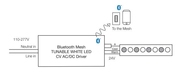
For best results, drivers need to be installed within 30 feet of the closest device within the Bluetooth Mesh network. Signal strength significantly decreases in presence of metal barriers such as when devices are enclosed in metal boxes.
