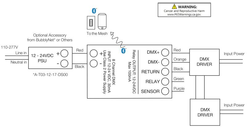
The relay must be protected against inductive over voltage spikes, ie. it must have a flyback diode. Do not connect a typical PCB relay without the diode.
